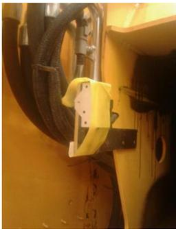
The picture attached shows the tape and metal in place. When removed the machine functioned correctly.
